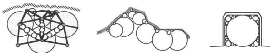
figure 3 : a model of agglomerate : mobile body and rigid (ground type) fixed obstacles.
