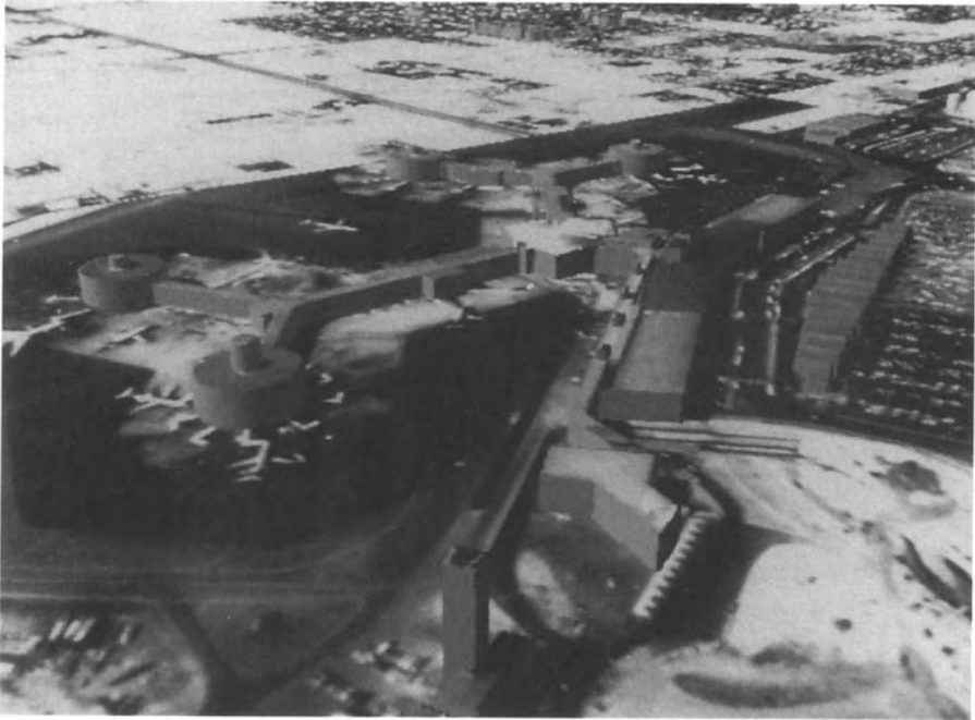
Figure 3: A volumetric model of an airport enhanced with photo-mapping of satellite images. The buildings are synthetic voxel models raised on top of the terrain.
