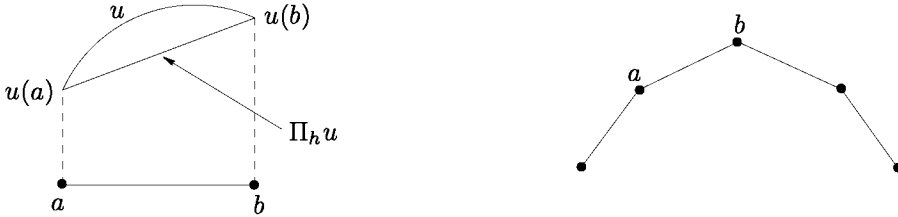
Figure 10.6: Piecewise linear interpolation in one dimension. Left-hand side: the segment I = [a, b] , u(a) and u(b) , the function \Pi_h u , the segment [u(a), u(b)] and the presumed function u . Right-hand side: the segment ab and its neighbors.
