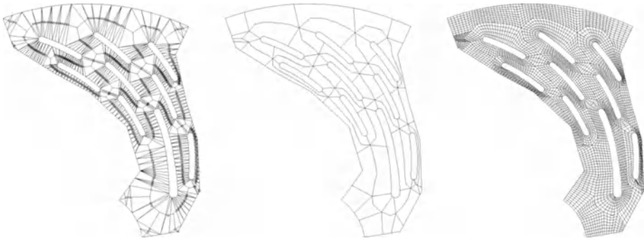
Figure 9.14: Examples of quad meshes based on the medial axis, in two dimensions: Delaunay triangulation of the domain (left-hand side), domain partitioning using the approximated medial axis (middle) and domain mesh resulting from an algebraic method (right-hand side).
